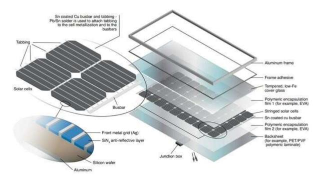
Other materials in the solar cells may be more difficult to recycle. Silver and copper are valuable components, but panels typically contain very small amounts of these materials. Toxic metals like lead and cadmium may also be present in solar panels.
