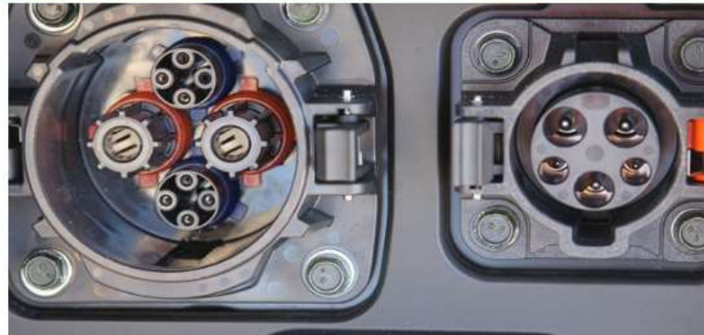
CHAdeMO DC and J1772 AC, Alternative Sockets as Mounted in the Nissan Leaf
